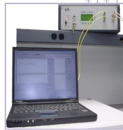
Signals sent out to optics via fiber optic cables and return to analyzer via coaxial cables. Data is displayed on a networked laptop.
